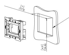
1. CUT OPENING - BOARD THICKNESS 10mm [0.39"]
