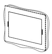
TO OPEN THE SCREEN, REMOVE THE BEZEL AND PULL OUT THE SCREEN  $\,$
