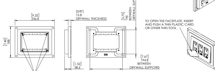
by Wall-Smart www.wall-smart.com LINLESS OTHERWISE SPECIFIED: DIMENSIONS ARE IN MILLIMETERS INFORMATION CONTAINED HEREIN IS PROPRIETARY AND MAY NOT BE USED, REPRODUCED OR COPIED WITHOUT WRITTEN CONSENT OF WALL-SMART ©
