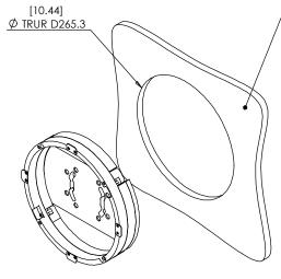
1. CUT OPENING - BOARD THICKNESS 10mm [0.39"] UP TO 22mm [0.86"] USE PAGE 3 FOR ROUTING TEMPLATE
