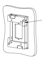
4. GENTLY SCREW-**CLOCKWISE 4 RETENTION** SCREWS UNTIL CAM LATCHES RETAIN THE UNIT
