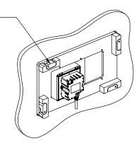
If required, it is possible to unscrew 6 screws, remove the back wall and connect
