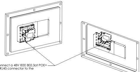
Before installation of the wall mount, connect a 48V IEEE 802.3at POE+power source via a CAT5/6 cable and RJ45 connector to the POE to USB converter.
