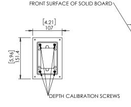
SOLID BOARD THICKNESS RANGE: 7.5 ~ 21.8 [0.3" ~ 0.86"] WITH SPACER ~ 33.1 [0.75" ~ 1.3"] WITHOUT SPACER [1.61]
