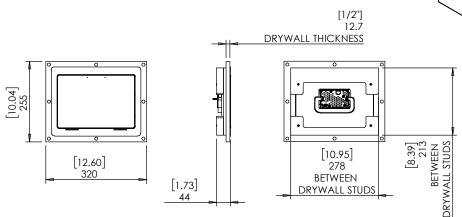
LINLESS OTHERWISE SPECIFIED: DIMENSIONS ARE IN MILLIMETERS
