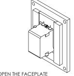
TO OPEN THE FACEPLATE INSERT AND PUSH A THIN PLASTIC CARD INTO THE VERTICAL GAP ON THE BOTTOM RIGHT OR ON THE TOP LEFT CORNERS
