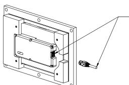
Before installation of the wall mount, connect a 48V IEEE 802.3at POE+ power source via a CAT5/6 cable and RJ45 connector to the POE to USB converter.
